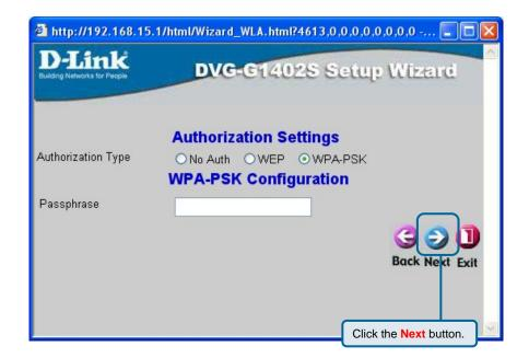
WPA-PSK (Pre-Shared Key) uses the same encryption as WPA but is implemented differently. All devices on the wireless network share the same key (a Passphrase). Enter the Passphrase in the field above.
